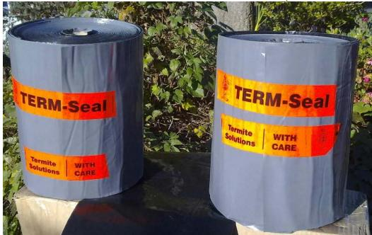
TERM-seal Ura-Fen Shield TDB is a sheet termite, moisture and damp-course barrier to be installed into buildings, that comprises a top and bottom untreated polyolefin cover sheets with an active matrix sheet of open cell polyurethane foam that contains 2gm/kg Bifenthrin as the active constituent. Ura-Fen Shield can be installed as a complete termite and moisture barrier under concrete slabs, across cavities as a building perimeter barrier, joints and penetrations or as an ant capping.
